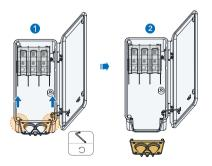
4. Loosen the four screws on the sealing plate with a wrench and remove the five-hole cable entry plate. Please properly store the four screws that are removed, which will be used in step 5.
