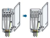
11. Remove the limit rod and place it in place. Close the junction block and tighten the two screws on its front cover with the hexagon socket wrench provided.
