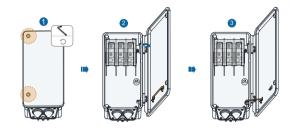
3. Loosen the screws on the bottom sealing plate with the hexagon socket wrench provided and remove the bottom sealing plate.
