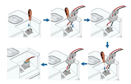
4. Fix the power connector with screws.
