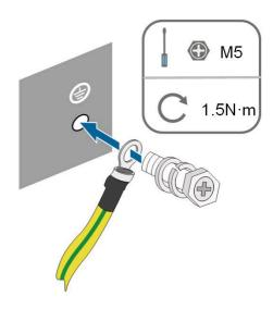
3. Apply silicone or painting to the PE terminal for corrosion protection.
