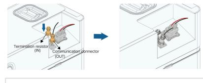
Be sure to install a termination resistor, otherwise, the battery communication cannot be enabled.
