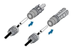
5. Fit the swivel nuts onto the connectors and tighten them. Pull gently the cables backward to make sure the connection is secure.
