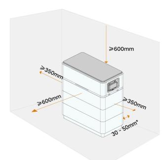
\* This distance is the distance between the RACK and the wall.
