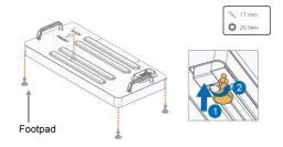
step 2 Mark the locations of holes for installing the battery fixing bracket. Position the base with its back against the wall, mark the installation position of the battery fixing bracket, and then move the base away.
