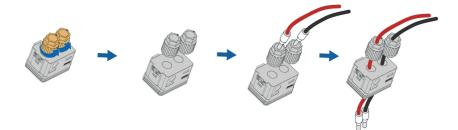
3. Insert the slotted screwdriver straight into the DC port, and press down on the screwdriver. The cable terminals can now be inserted into the corresponding ports. Release the pressure on the screwdriver, and the DC cables will be secured automatically.
