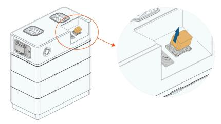
2. On the battery side, lead the DC cables through the power connector.
