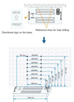
Reference lines for hole drilling: Used for determining the spacing between the two holes at the ends of the battery fixing bracket.
