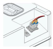
3. On the battery side, pull the DC cables out directly.
