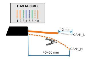
3. Insert the stripped wires into the corresponding cold-pressed terminals, and crimp them using a crimping tool.
