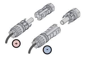
6. Pull gently the DC cables backward to check whether the connection is secure.
