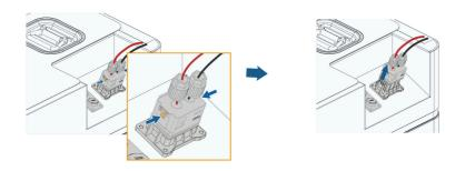
4. On the inverter side, loosen the locking element of the connector with a dismantling wrench, and fit the waterproof plug.
