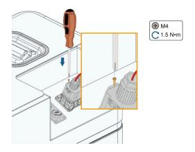
5. On the inverter side, connect the connectors of the DC cables to the corresponding BAT terminals of the inverter, and make sure they "click" into place.
