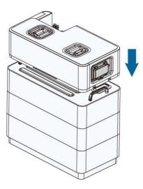
step 8 It is needed to install the switch gear fixing bracket, so as to prevent arc faults caused by moving the switch gear by mistake. Insert the bracket into the gap between the switch gear and the PACK, and fix it using screws.
