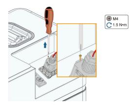
2. Rotate anticlockwise the waterproof terminals at the end of the connector.
