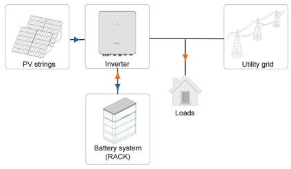
figure 2-1 System Diagram
