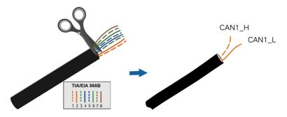
2. Remove the insulation of the signal wires, both by 12mm.
