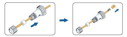
3. Attach the RJ45 connector, and crimp it using the RJ45 crimping tool.
