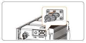
Figure 7-60 Installing the WiFi connecting cable
