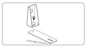
Figure 6-7 Attaching two brackets
