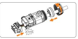
Figure 7-24 Assembling the AC connector
