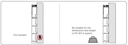
Figure 4-5 Installation carrier requirement
