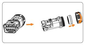
Figure 7-18 Disassembling the AC connector
