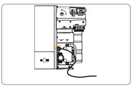
Figure 12-8 Disconnecting the CT/Meter cable
