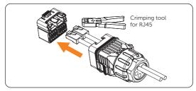
**Step 3:** Crimp the stripped end with RJ45 terminals with a crimping tool for RJ45.
