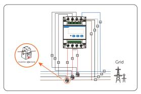
Figure 14-11 Connecting CT-connected meter to the grid
