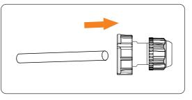
Figure 7-42 Threading the communication cable
