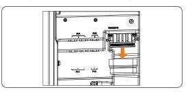
Figure 7-26 Removing the dustproof cover
