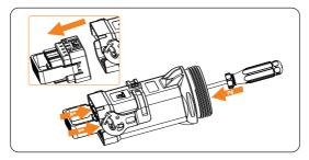
Figure 7-21 Poking the rubber core out
