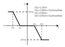
Figure 9-51 Curve Q=f(V)
