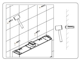
Figure 6-20 Knocking expansion tubes into the wall
