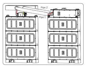
Figure 7-11 Inserting pipes into the cover
