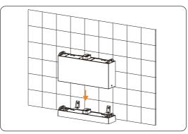
Figure 6-12 Placing the battery module
