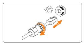
Figure 7-47 Connecting cable to the CT/Meter port
