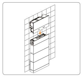
Figure 6-26 Installing the inverter
