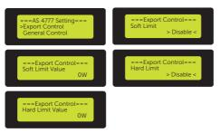
Figure 9-60 Setting export control in AS4777 setting interface
