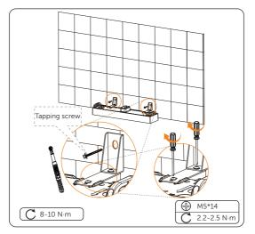
Figure 6-11 Securing the assembled bracket
