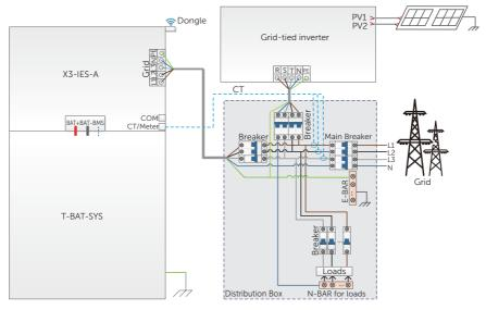
Figure 2-25 System diagram with grid-tied inverter for Australia
