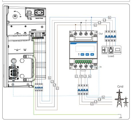
Figure 14-5 System wiring with direct-connected meter
