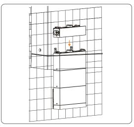
Figure 6-47 Placing the BMS
