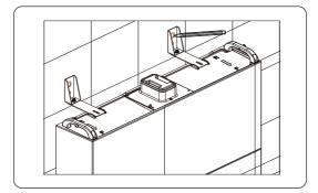
Figure 6-16 Marking the position of BMS
