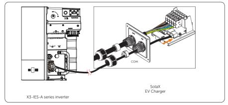
Figure 7-30 Inverter connected with a SolaX EV Charger
