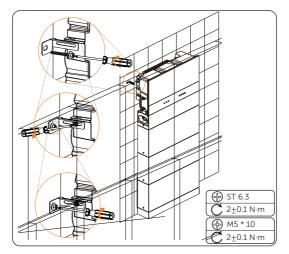
Figure 6-28 Locking the inverter brackets
