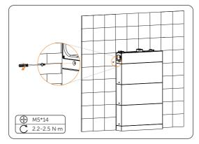
Figure 6-23 Tightening M5 screws
