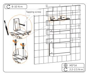
Figure 6-46 Securing the assembled bracket
