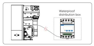
Step 3: Connect the conductors to terminal 24 and 25 of the meter.
