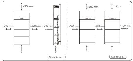
Figure 4-6 Clearance requirement
