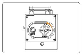
Figure 12-2 Turning off the BAT switch
