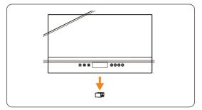
Figure 6-25 Removing the dustproof cover
