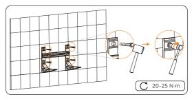
Figure 6-35 Tightening expansion screws
