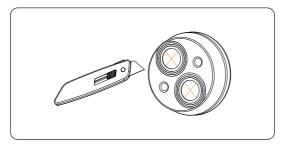
Figure 7-19 Cutting the round membrane
