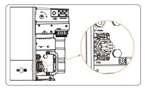
Figure 7-32 Well connected COM port
