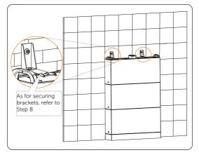
Figure 6-21 Tightening the BMS brackets
