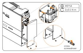
Figure 7-50 Locking the cable shielding board
