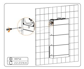
Figure 6-48 Tightening M5 screws
