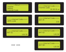
Figure 9-90 Displaying the internal code information
