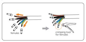
Figure 7-17 Crimping the Grid cables
