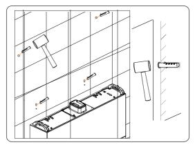
Figure 6-45 Knocking expansion tubes into the wall
