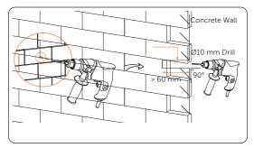
Figure 6-9 Drilling holes
