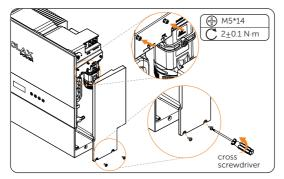
Figure 7-48 Locking the cable shielding board
