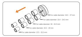
Figure 7-20 Taking out sealing plug
