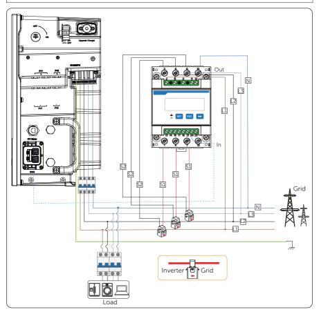
Figure 14-10 System wiring with CT-connected meter
