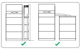
Figure 6-1 Correct installtion angle
