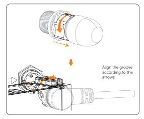
Figure 7-12 Locking heater cable
