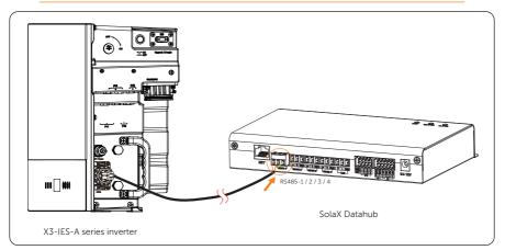
Figure 7-29 Inverter connected with a SolaX datahub
