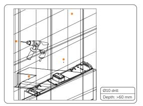
Figure 6-44 Drilling holes
