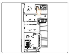
Figure 8-3 Pressing the inverter button
