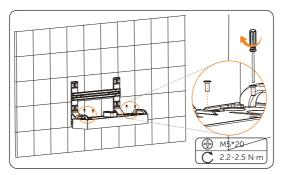
Figure 6-36 Securing the base
