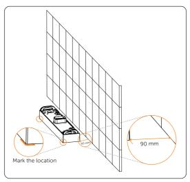
Figure 6-6 Placing the base
