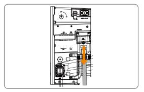
Figure 12-5 Unplugging the AC connector
