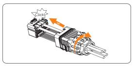
Figure 7-39 Inserting the terminal block into the connector
