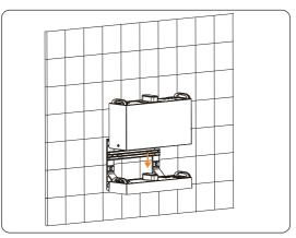
Figure 6-37 Placing battery module
