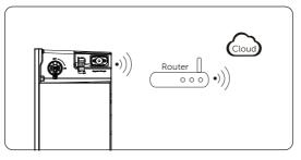
Figure 7-53 WiFi mode connection diagram
