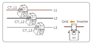
Figure 14-2 Clipping CTs to grid cables
