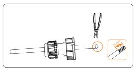
Figure 7-45 Stripping the communication cable for meter
