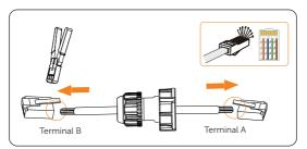
Figure 7-44 Crimping the communication cable for CT
