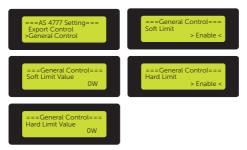
Figure 9-61 Setting general control in AS4777 setting interface
