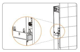
Figure 7-52 Installing the padlock
