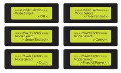
Figure 9-43 Selecting a mode in power factor
