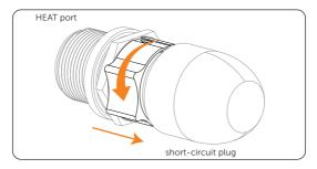
Figure 7-8 Closing short-circuit plug
