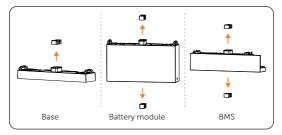
Figure 6-31 Removing dust covers
