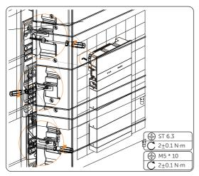
Figure 6-53 Locking the inverter brackets
