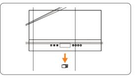
Figure 6-50 Removing the dustproof cover
