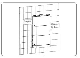
Figure 6-39 Placing battery modules
