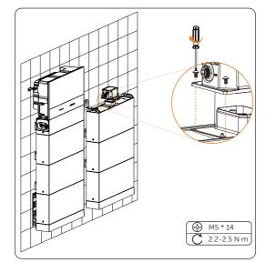
**Step 2:** Place the series box, insert and tighten M5\*14 screws, with totalling 4 screws (torque: 2.2-2.5 N·m).
