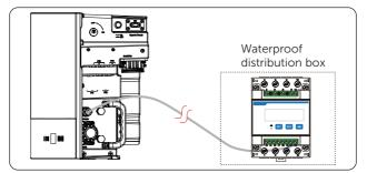
Figure 14-13 Connecting inverter to meter
