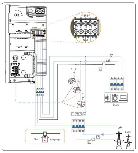
Figure 14-1 System wiring with CT
