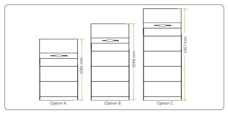
Figure 4-3 Installation options for one tower
