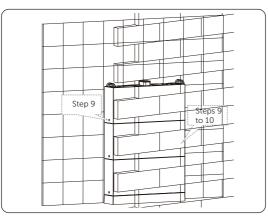
Figure 6-14 Placing battery modules
