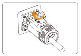
Figure 12-4 Removing the latch of the AC connector
