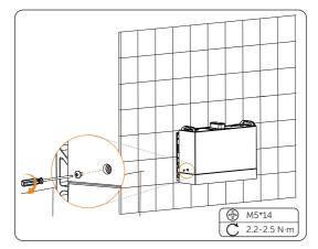
Figure 6-38 Tightening screws
