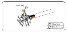
Figure 7-23 Locking wires in the AC connector
