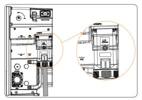
Figure 7-15 Well connected Grid cables
