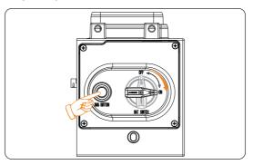
Figure 8-2 Turning on the battery
