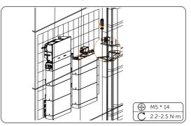
Figure 6-30 Placing the series box
