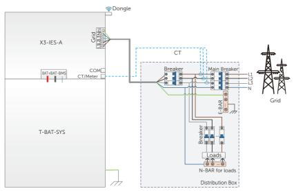
Figure 2-22 System diagram without grid-tied inverter for most countries
