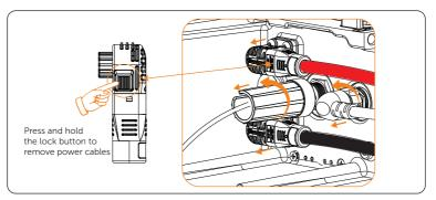
Figure 12-10 Disconnecting battery connectors
