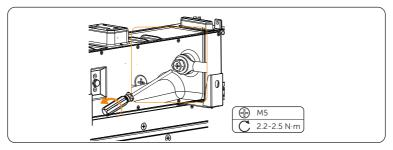
Figure 12-11 Disconnecting grounding cable
