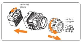
Figure 7-33 Disassembling the communication connector
