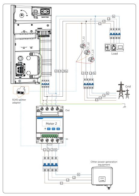
Figure 14-15 Connection diagram of CT and direct-connected meter
