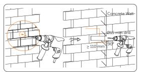
Figure 6-34 Drilling holes
