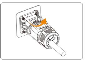
Figure 12-3 Loosening the AC connector
