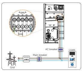
Figure 8-1 Turning on AC breaker
