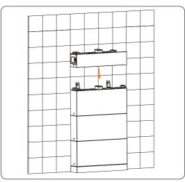
Figure 6-22 Placing the BMS
