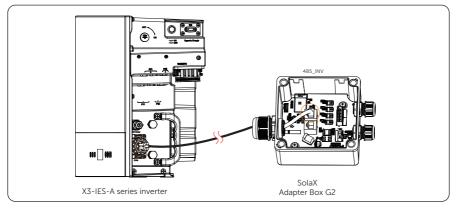
Figure 7-31 Inverter connected with a SolaX Adapter Box G2
