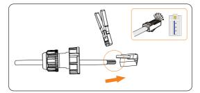
Figure 7-46 Crimping the communication cable for meter
