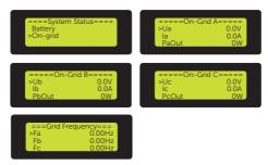
Figure 9-15 Displaying on-grid status
