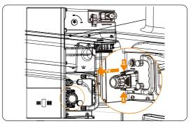
Figure 12-7 Disconnecting the communication connector
