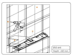
Figure 6-19 Drilling holes
