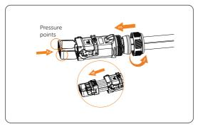
Figure 12-6 Poking the terminal block out of the AC connector
