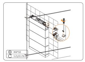
Figure 6-49 Install the anti-tamper bracket
