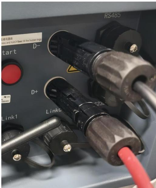
**Battery side: Connect power cables.**
